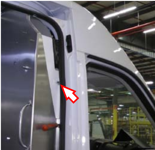
Fastener in upper B-pillar
