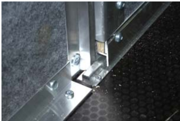
Door track to RH front floor angle alignment
