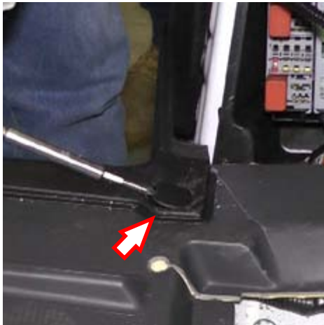
RH stepwell liner screw and cover
