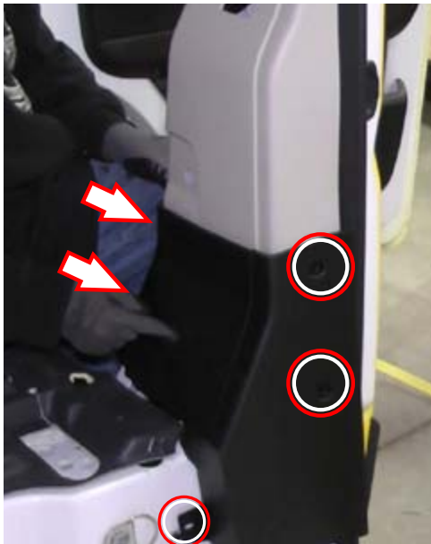
Lower B-pillar trim fasteners
